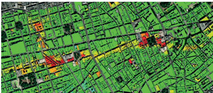
The figure shows the impact of tunneling works on nearby buildings. Risk Index for single building is provided. Images TerraSAR-X © Airbus
