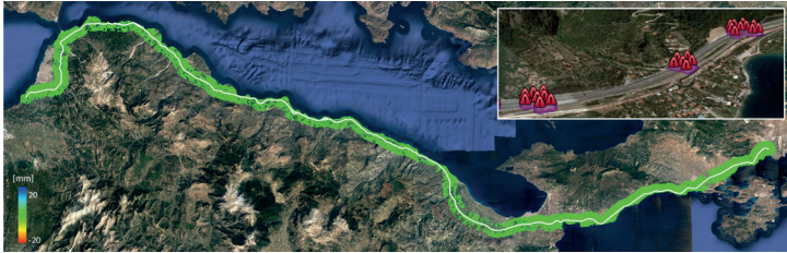
The figure above shows 2 years of accumulated deformation on 200 km of motorway, and the filtering of areas affected by active deformation. Images Sentinel-1 ©ESA
